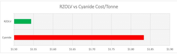
Based on 30-day comparable flooded column leach tests on RV Mine oxidized ore – vs 1,000 PPM NaCN
